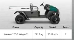
Delivers the power, and strength of a 4-wheel drive vehicle with even higher payload capacity. Features 4-wheel disc rakes and tows up to 680.3 kg [4]
